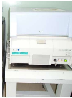
XRF (HITACHI Highttech SEA-1200VX Measurement range: _{11}\text{Na} to _{92}\text{U} )
